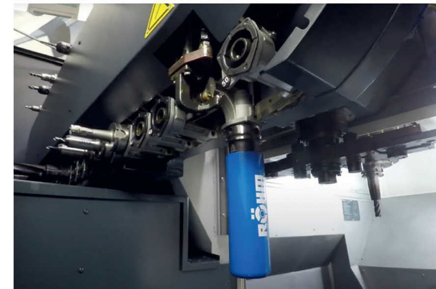
The Lubritool has is stored ready for use in the tool changer and is simply swapped automatically for the lubrication operation by the machining program
