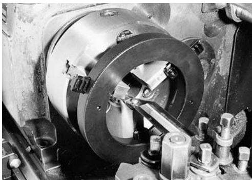
Turning the inside diameters of soft jaws
