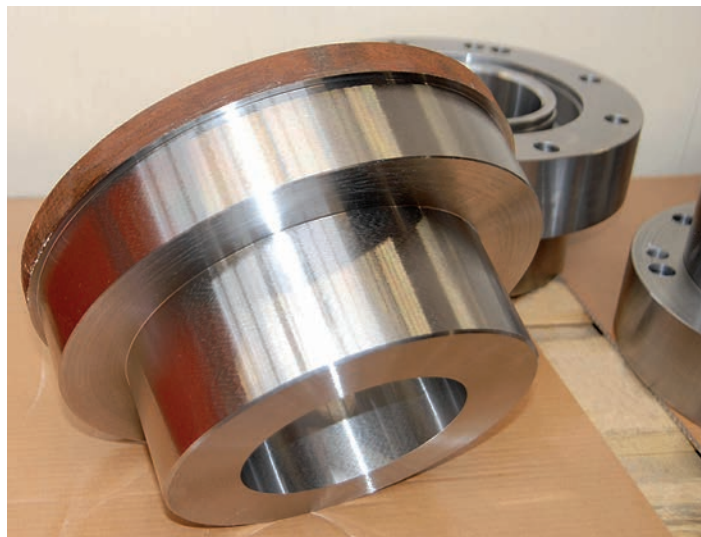
With just two easily effected clamping operations, unfinished parts weighing up to 550 kg can be processed into precise slide bearings, flanges and spiral gaskets for high-efficiency pumps.
