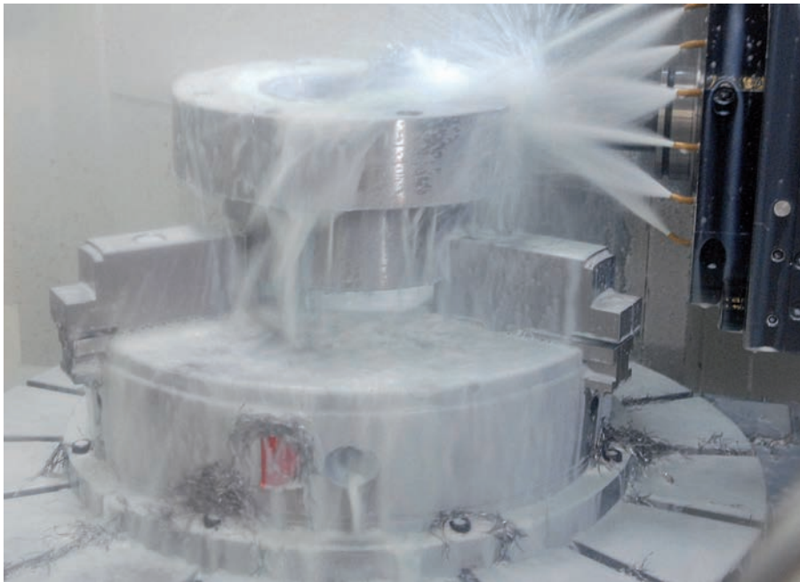
The concentric and axial runout accuracy of the DURO-T is twice as good as that required for DIN Accuracy Class 1.
